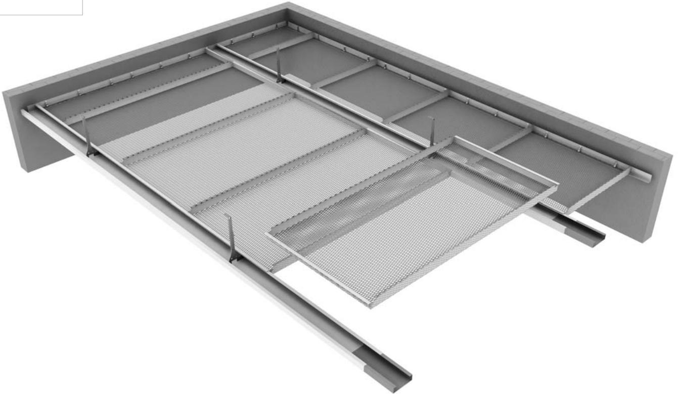
Integra Expanded Perspekta Bandraster Systems provide architects with modern application alternatives. The system is formed with C or D Bandraster (50 – 100 – 125 – 150 – 200) which allow the system to be easily demounted without the need for tools.
